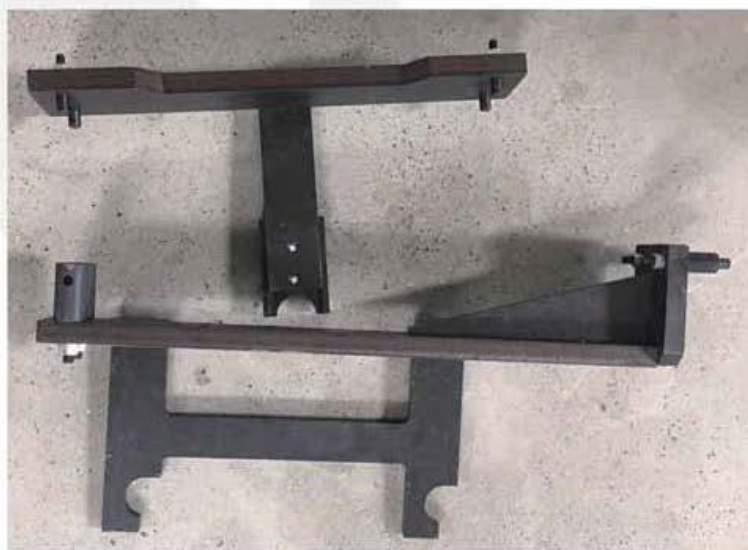
Calliper for driving shaft 转动轴卡板
